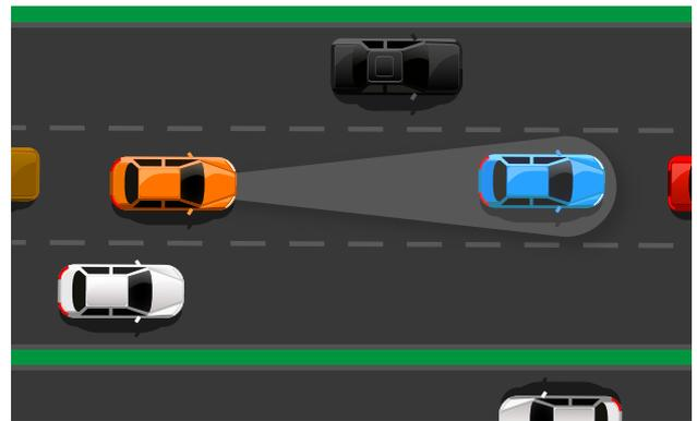
Switch on the adaptive cruise control and put in the maximum speed you want to drive and the distance at which you're comfortable following other cars. As long as there's no one in front of you the car will maintain that speed without any driver input. When you inevitably come across a slower vehicle, or even stop and go traffic, the vehicle will automatically brake and accelerate to keep up with traffic.
