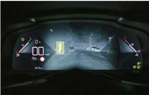
An automotive night vision system uses a thermographic camera to increase a driver's perception and seeing distance in darkness or poor weather beyond the reach of the vehicle's headlights. This may help to highlight humans and other objects that wouldn't otherwise be seen as clearly with just normal vehicle headlights. Such systems are offered as optional equipment on certain premium vehicles.
