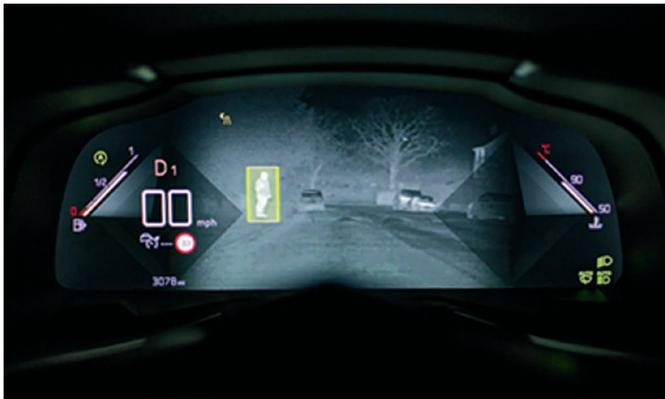
An automotive night vision system uses a thermographic camera to increase a driver's perception and seeing distance in darkness or poor weather beyond the reach of the vehicle's headlights. This may help to highlight humans and other objects that wouldn't otherwise be seen as clearly with just normal vehicle headlights. Such systems are offered as optional equipment on certain premium vehicles.
