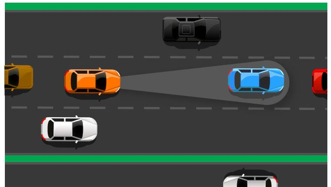
Switch on the adaptive cruise control and put in the maximum speed you want to drive and the distance at which you're comfortable following other cars. As long as there's no one in front of you the car will maintain that speed without any driver input. When you inevitably come across a slower vehicle, or even stop and go traffic, the vehicle will automatically brake and accelerate to keep up with traffic.
