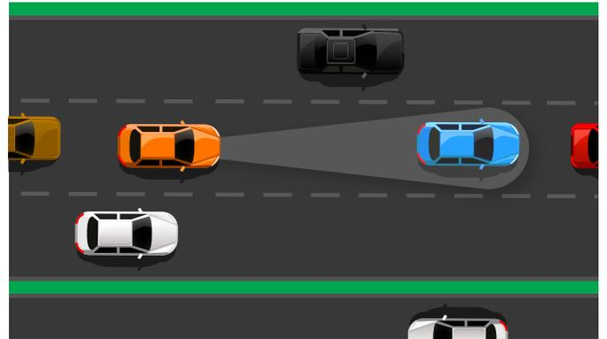
Switch on the adaptive cruise control and put in the maximum speed you want to drive and the distance at which you're comfortable following other cars. As long as there's no one in front of you the car will maintain that speed without any driver input. When you inevitably come across a slower vehicle, or even stop and go traffic, the vehicle will automatically brake and accelerate to keep up with traffic.
