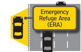
Smart motorways have ERAs spaced at regular intervals. They have cameras, not always detection technology.
